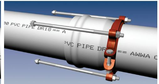
4. Remove the side bolts from the serrated restraint ring. Use the tie bolts to determine the proper location of the restraint ring on the spigot. Allow enough room on the tie bolt to fully engage the nuts.
