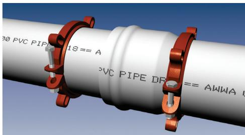
5. Install both halves of the restraint ring at the proper location, tapping each half into place. Make sure that the complete ID of the ring is touching the pipe before installing the side bolts. Tighten the side bolts evenly to 60 ft-lbs torque (110 ft-lbs on 8 inch, 10 inch and 12 inch).
