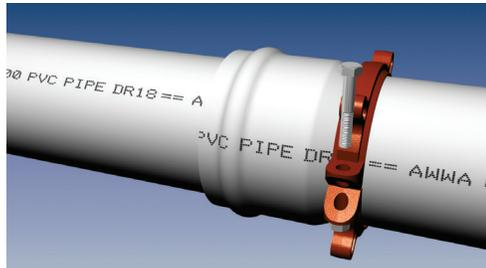
2. Install both halves of the non-serrated bell ring around the pipe behind the bell. Install the side bolts and tighten each to 60 ft-lbs (110 ft-lbs on 8 inch, 10 inch and 12 inch).
