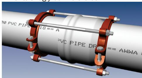
6. Place nuts on the tie bolts and tighten until they are snug. Allow enough room on the tie bolt to fully engage the nut with several threads showing. Do not tighten these bolts enough to force the spigot further into the bell of the joint.
