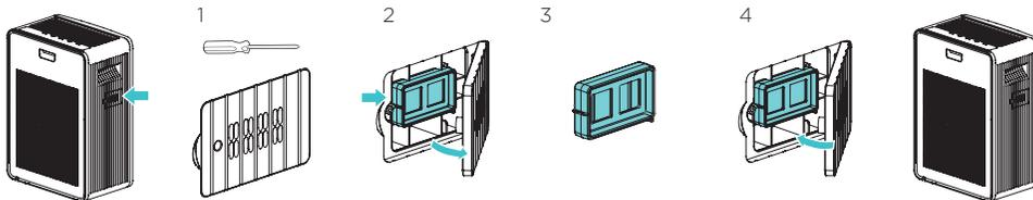
For accurate air quality display readings, the blue sensor screen should be gently cleaned with a cotton swab once every two weeks.
