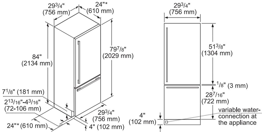
\*Excludes thickness of door panel. If standard panel with 3/4" thickness is mounted, total depth is 24 3/4".
