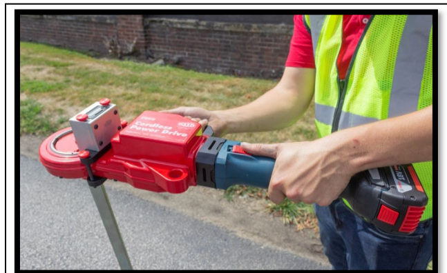
CPDWW powers valve turning with VOKUCLUTCH Utility Clutch and CPDWWCNT Digital Counter
