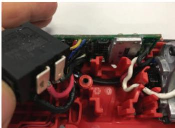
**NOTE:** Be sure to place all components of the Electronics Assembly (64) firmly and squarely in Left Housing Halve-Support (55). Be sure to route wires into wire traps as shown. Check for any interferences prior to installing the Housing Cover (51).
