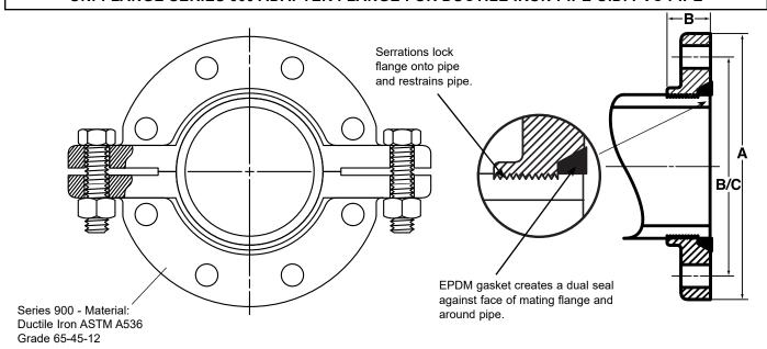
Color Code: Red for PVC with ductile iron pipe O.D.
