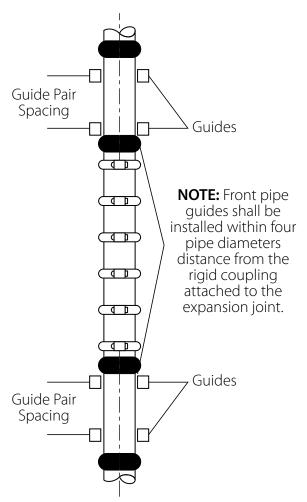
Guide pair space requirements: Minimum = 12 pipe diameters Maximum = 14 pipe diameters
