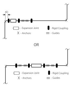
At the system designers option, some long straight pipe runs may require additional guides to maintain pipe alignment and prevent "bowing" and pipe joint deflection on areas remote from the expansion compensation device. The use of Victaulic rigid couplings with proper pipe support spacing (see <a href="mailto:publication26.01">publication26.01</a> for additional information) may eliminate the need for the additional guides.
