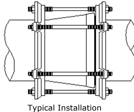
**3. INSTALL BELL RING:** Assemble one set of ring segments behind the bell. Adjust ring to suitable diameter, and lock ring segments into position by tightening nuts.
