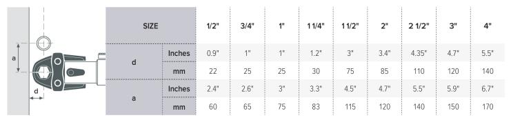
Tab. 3 - Minimum depths of the pipelines installed in-wall.
