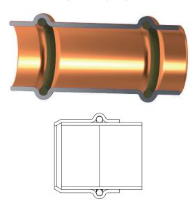
FNW Copper Press Fittings (from 2-1/2" to 4") feature an XLC profile designed for maximum safety. An internal steel gripping ring (placed upstream of the O-ring and following the direction of insertion of the pipe) grips into the tube when the joint is pressed, creating a durable and safe joint. A nylon separation ring, placed between the gripping ring and the O-ring, protects the sealing element, making the pipe insertion operation safer.
