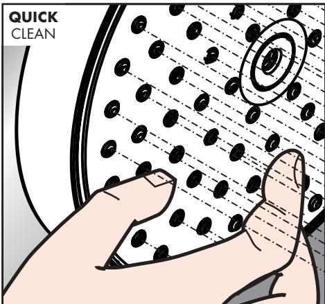
**JUST CLEAN:** simply rub over the spray nozzles to remove lime scale.
