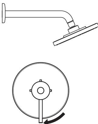
It is normal for the showerhead to drip for several minutes after the water is turned off. Water left in the showerhead is draining away. IT DOES NOT MEAN THAT THE SHOWER VALVE IS LEAKING.
