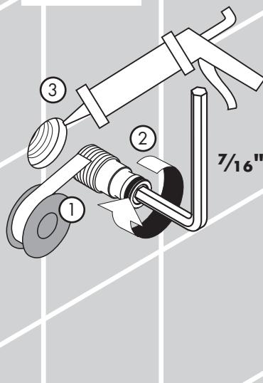
**3/4" NPT installation:** Wrap the mounting piece with plumbers' tape. Install the mounting piece.
