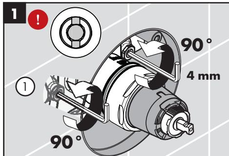
If the valve opens through hot, reverse the cartridge.
