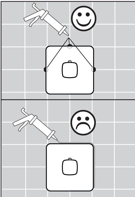
Place a dab of waterproof sealant at the grout joints.
