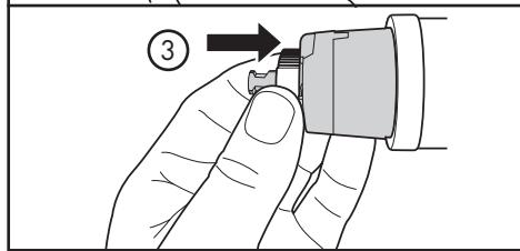
The temperature change per notch may be anywhere from 4° - 16° F, depending on local inlet conditions. Repeat as necessary.
