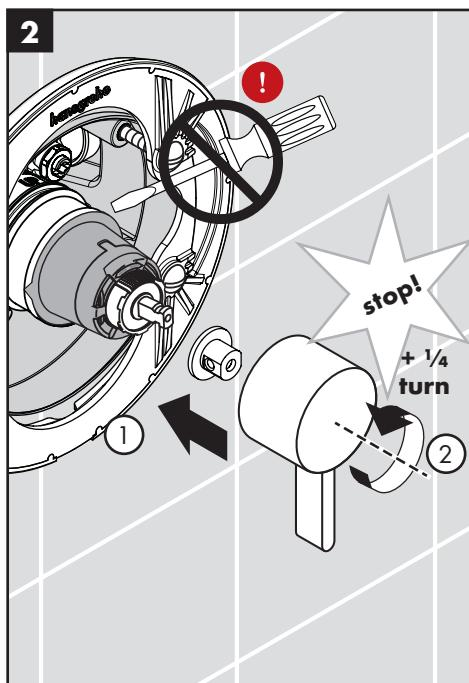
**⚠ Do not attempt to pry the cartridge from the function block by using a screwdriver. Damage to the cartridge will result.**
