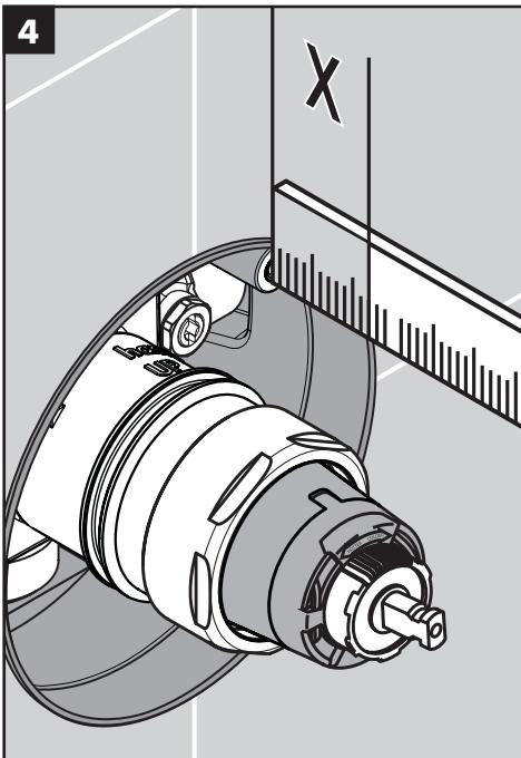
Measure the distance from the front of the plaster shield to one of the screw-in flanges ("X").
