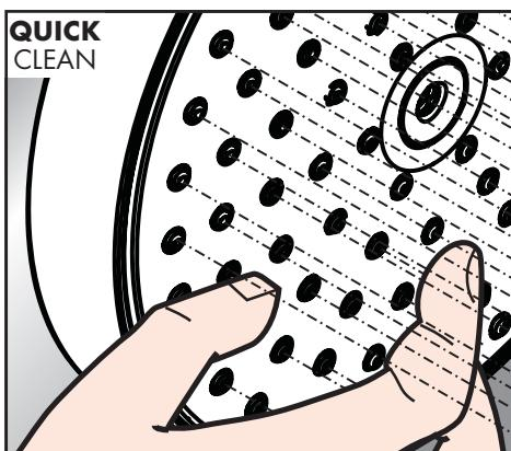
JUST CLEAN: simply rub over the spray nozzles to remove lime scale.
