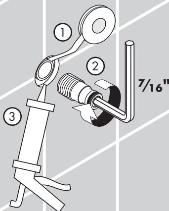
**1/2" NPT Installation:** Wrap the threads on the nipple with plumbers' tape. Install the mounting piece.
