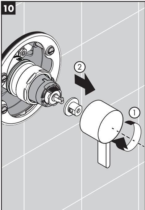
Turn the water off. Remove the handle and the adapter.
