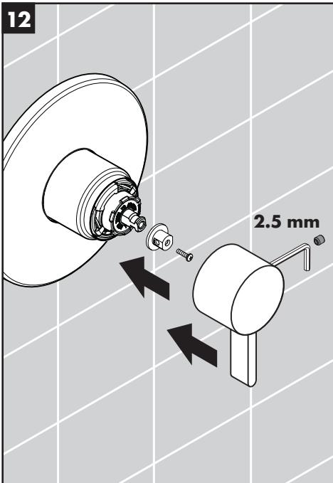
Install the handle adapter and the screw.
