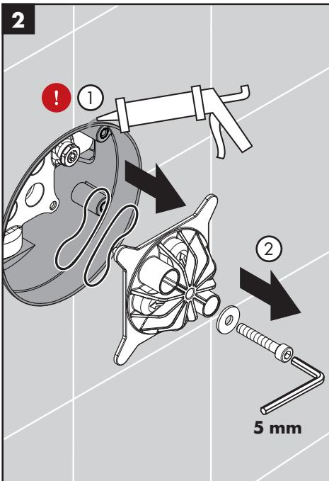
Seal the wall around the plaster shield with waterproof sealant.
