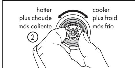
Rotate clockwise to decrease the maximum temperature. Rotate counter-clockwise to increase the maximum temperature.
