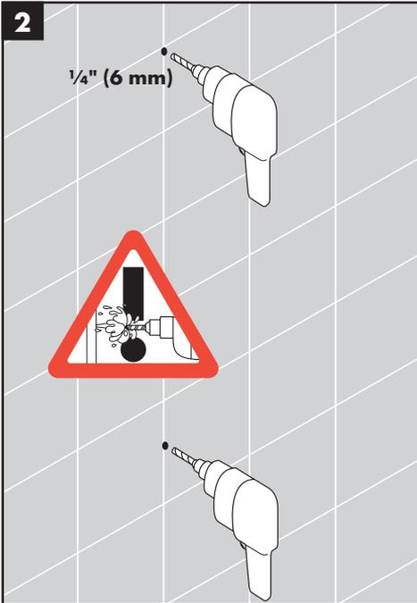
Drill the holes using a 1/4" (6mm) bit.
