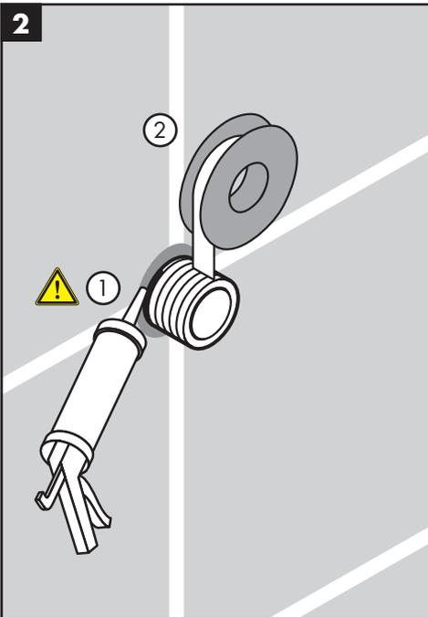
Seal the wall around the nipple with waterproof sealant.
