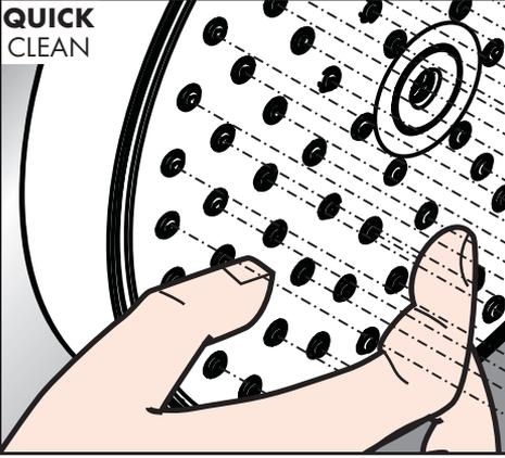
**Just clean:** simply rub over the spray nozzles to remove lime scale.
