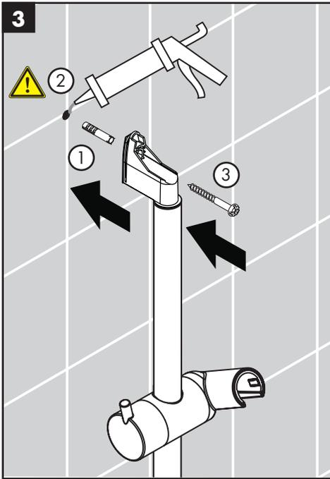
Install the anchors. Seal the wall around the anchors with waterproof sealant.
