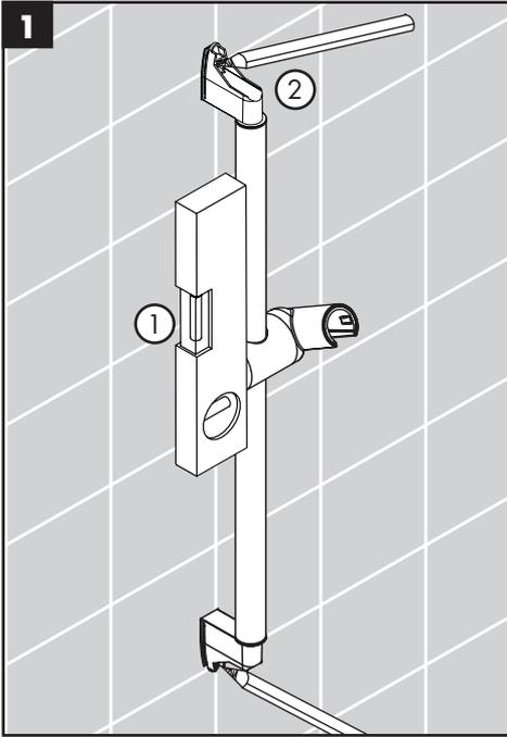
Place the bar against the wall at the desired mounting location. Make sure that it is level.
