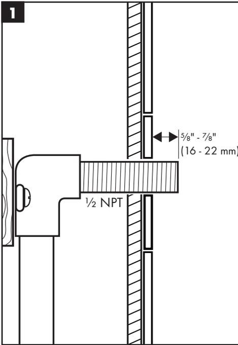
Install a NPT 1/2" male threaded nipple, extending 5/8" - 7/8" (16 - 22 mm) outside the surface of the finished wall.
