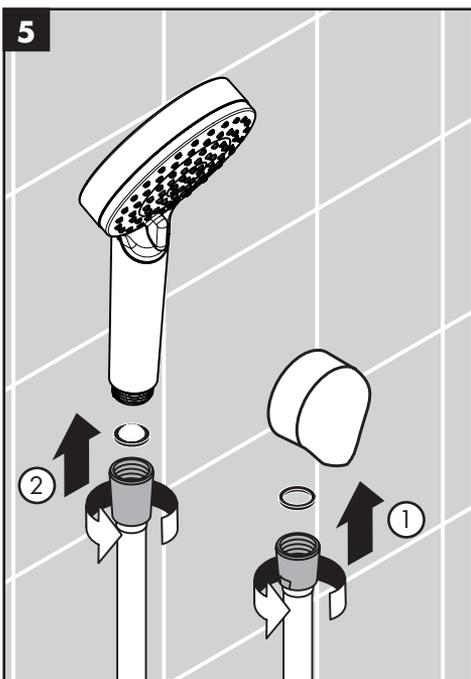
Place a black rubber washer in the short end of the handshower hose. Connect this end to the wall supply.
