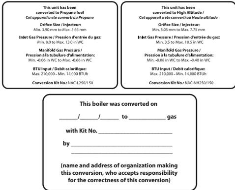
Figure 11. Proper Placement of Propane Gas or High Altitude Conversion Labels
