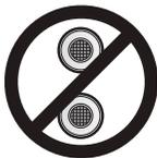
Do not vertically stack concentric terminations on sidewalls.
