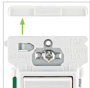
Longer and wider strap is compatible with Midway wallplates, and with Standard sized wallplates when breakaway tab is removed
