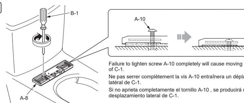
Failure to tighten screw A-10 completely will cause moving sideways of C-1.
