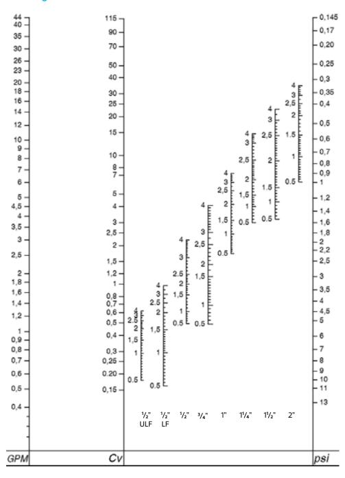
Using diagram, determine the presetting position of the valve with the given design flowrate and headloss:
