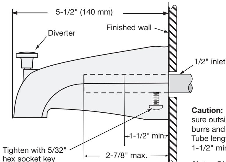
**Caution:** Ensure seal is not damaged by making sure outside of 1/2 inch diameter tube is free of burrs and sharp edges prior to tub spout installation. Tube length from finished wall should be 1-1/2" min. to 2-7/8" max.
