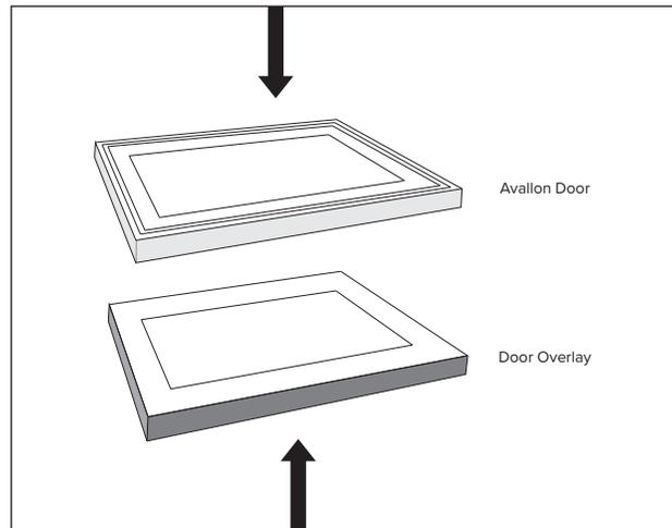
7. Drill pilot holes into your overlay panel using the screw hole openings in the Avallon door for exact placement.
