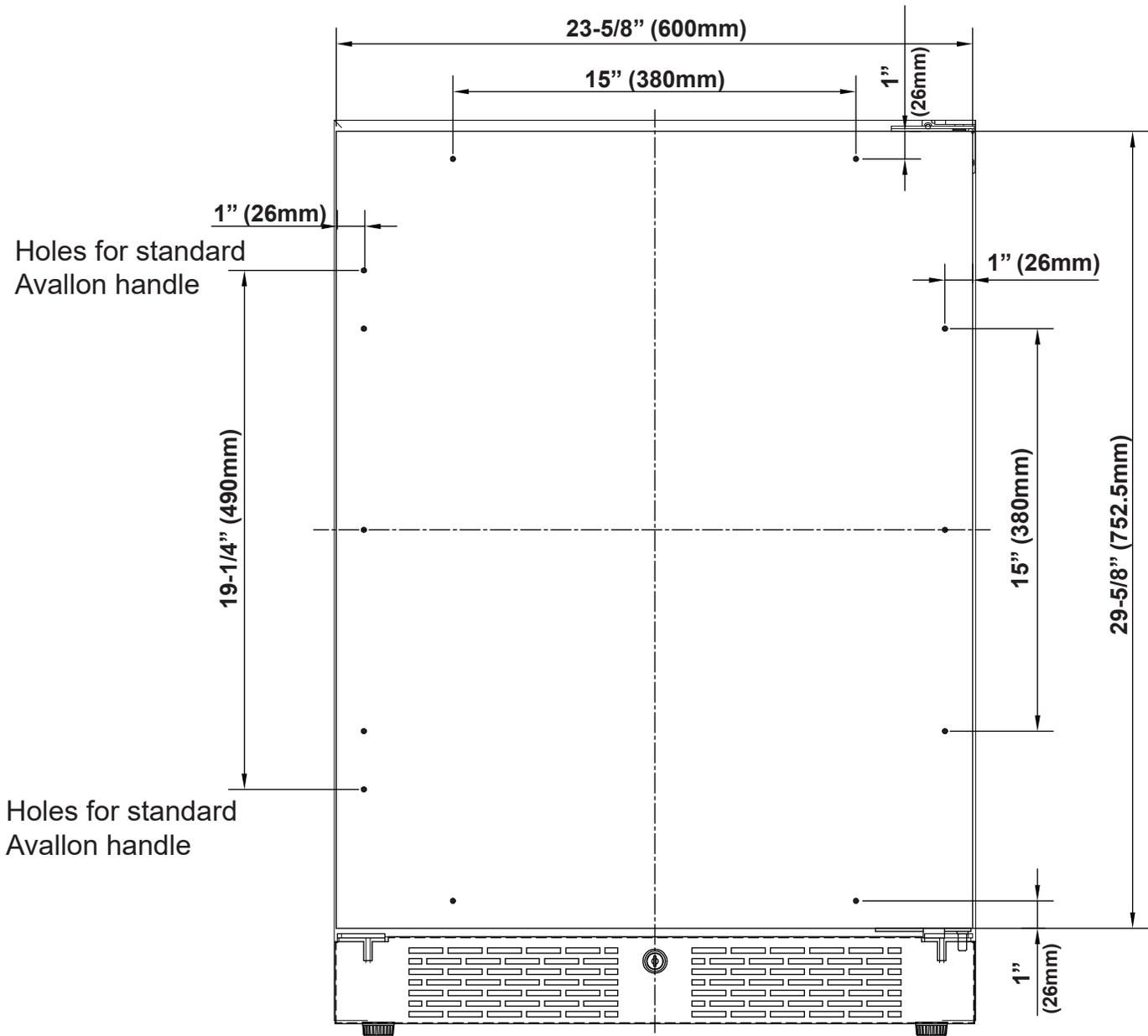
**\*Handle screw placement for left hinged models is reversed.**
