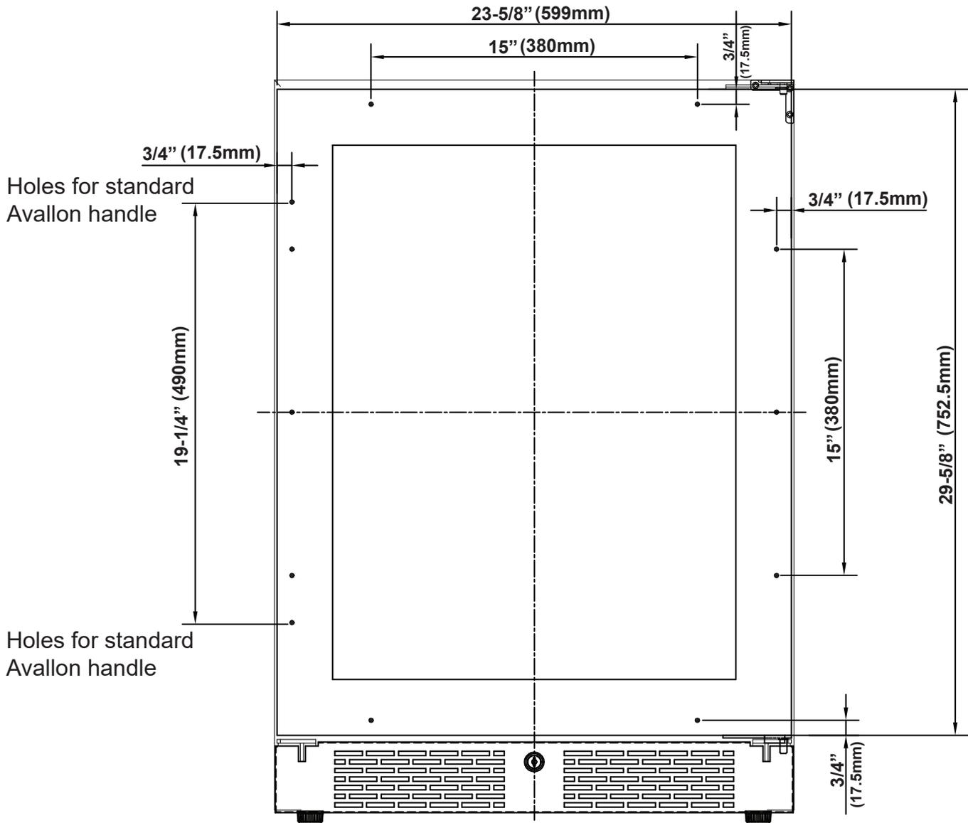
**\*Handle screw placement for left hinged models is reversed.**
