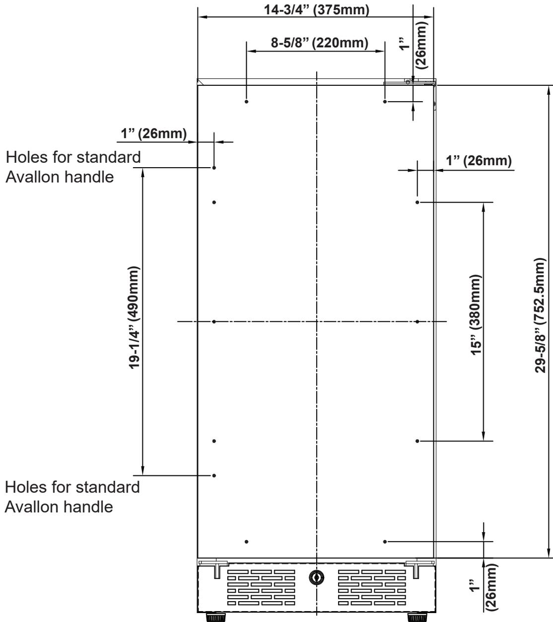
**\*Handle screw placement for left hinged models is reversed.**
