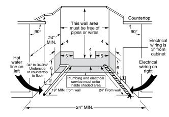
**Note:** Dishwasher must not be installed more than 10 feet from sink for proper drainage. All plumbing and electrical work must be in accordance with local codes. Dishwasher includes drain hose and leveling legs.
