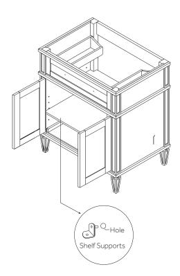
2. For added stability the shelf can be attached to the shelf supports using the provided screws. The bottom drawer will need to be removed to insert screws into shelf supports. The drawer can be removed by squeezing release clips on underside of the drawer.
