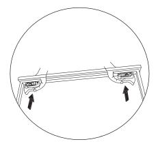
2. Remove the screw from the shelve supports if needed. Lift up the shelve and reposition the shelf supports to the desired height. Rest the shelve on the shelve supports and reinstall screws (if desired).
