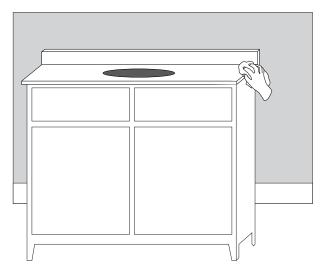
3. If you are installing a side-splash and/or back-splash, place a generous amount of silicone sealant on the back of it and press it into place against your bathroom wall. Fill any gaps that are left with silicone sealant. Wipe away any excess sealant with a damp cloth.
