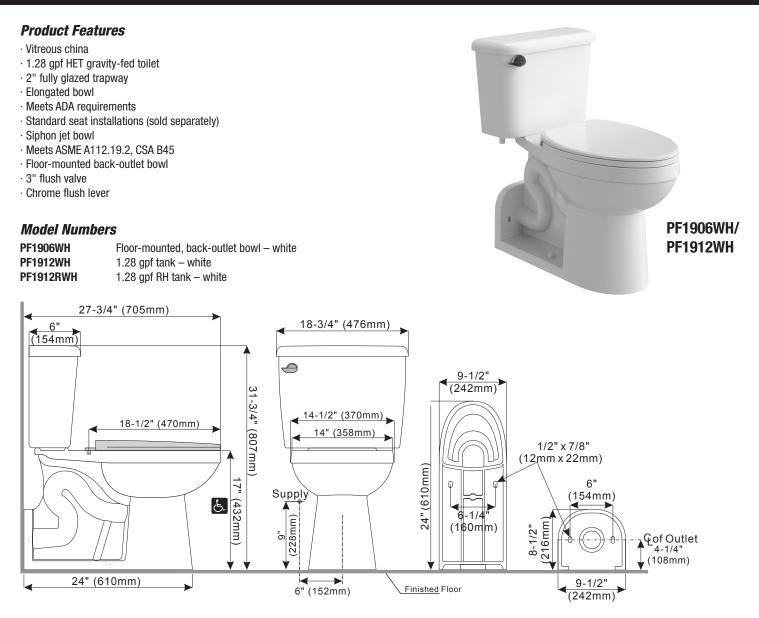
Note: All dimensions and specifications are nominal and may vary: Dimensions of 8" and greater have a tolerances of +3%. Dimensions less than 8" have a tolerances of +5%.
