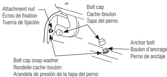
Snap bolt caps into place over the two anchor bolt heads and the two attachment nuts.
