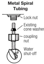
Use existing spiral cone washer. Fluid master cone washer may not seal completely on spiral type supply line.
