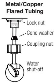
These parts must be used as illustrated to ensure water-tight connection. Use of existing coupling nut may result in water leakage. Water supply tube or pipe must extend at least 1/2" inside threaded shank of valve (does not apply to flanged tubing).
