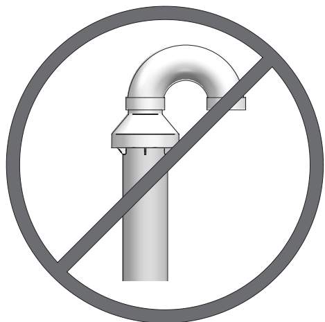
Figure 5-5 Do Not Install U-Bend to Rain Cap
