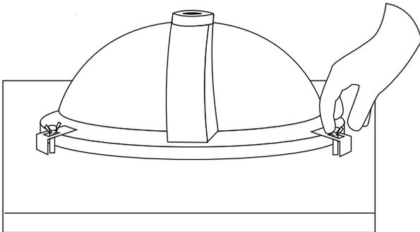
7. Carefully turn the countertop and sinks over. If needed, reposition the sinks by slightly loosening the wing bolts and adjusting.
