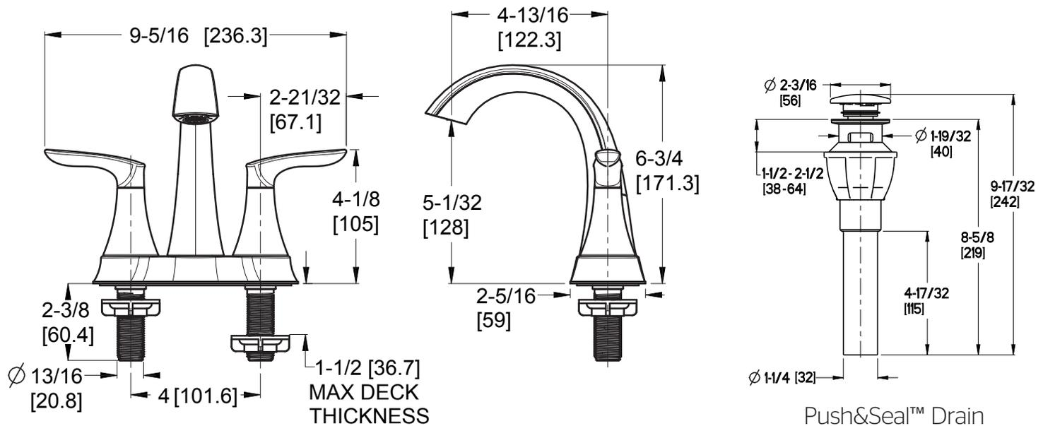
Ø1 Min to Ø1-1/2 Max. Deck Hole Openings
