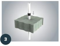
Slide wrap strip along the pipe and into the annular space as shown.
