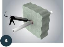
Apply caulking as required to close remaining gap to both sides of wall assembly; providing a smoke and gas resistant seal. Spread caulking smoothly and evenly all around.
