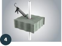
Apply caulking as required to close remaining gap to one side of floor assembly; providing a smoke and gas resistant seal. Spread caulking smoothly and evenly all around.
