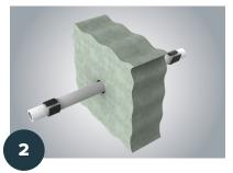
Apply wrap strips around plastic pipe for the specified number of times and fasten tightly using adhesive tape to both sides of wall assembly.
