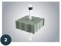
Apply wrap strip around plastic pipe for the specified number of times and fasten tightly using adhesive tape to one side of floor assembly
