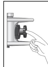
**WARNING:** Always lock the tool for carrying or moving to another anchor location. Grip the tool firmly when carrying.
