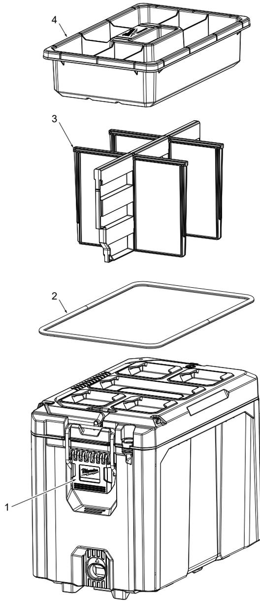
Note: Tray, Dividers and Gasket illustrated outside of PACKOUT, is to be assembled on the inside.
