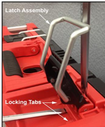
As an aid to removing a damaged Latch Assembly (9), use two large flat blade screwdrivers. Push blades between parts as shown. Twist both screwdrivers at same time to force the blades into opening and work the latch assembly over the two locking tabs.
