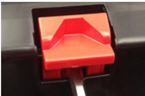
To remove a damaged locker system, flip tote over on the side and approach tote from the bottom of base. Insert a large flat blade screwdriver in middle of locking carriage as shown. Lightly pry carriage upward out of base opening. Remove and discard old locking carriage.
