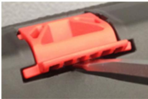
To remove a damaged locker system, flip tote upside down and approach tote from the bottom of base. Insert a large flat blade screwdriver in middle of locking carriage as shown. Lightly pry carriage upward out of base opening. Remove and discard old locking carriage and spring.
