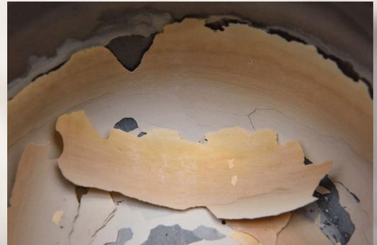
*Water heater with scale and sediment buildup decreasing the efficiency, water pressure and lifespan of this water heater.*
