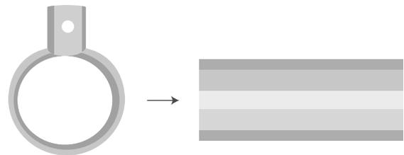
9. Insert the ends of the rod into the wall brackets. Tighten the set screws with a Philips head screwdriver to secure.
