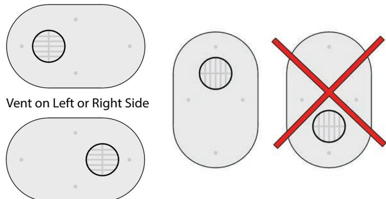
Figure 16 PVC low profile termination acceptable orientations
