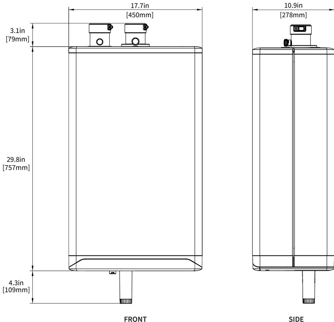
Figure 1a: Dimensions / Connections for **Tankless Water Heater**
