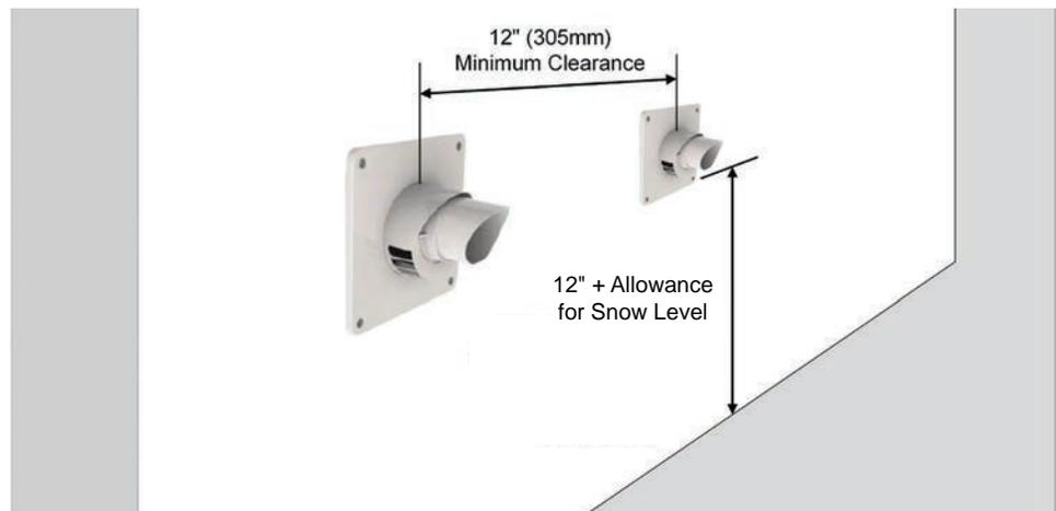
Figure 17: Horizontal Polypropylene Concentric Termination - Two Kits
