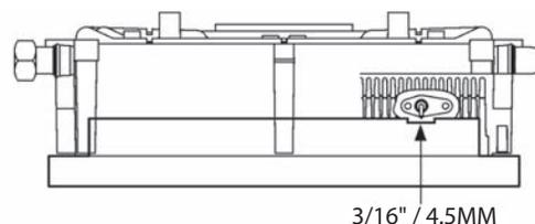
Figure 37: Checking igniter gap using 251-001 Ignitor Gapping Tool
