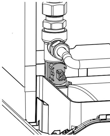
Figure 42: Domestic Hot Water Temperature Sensor S3
