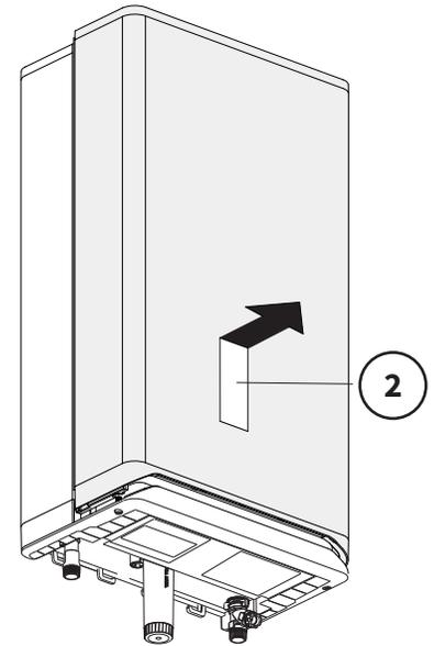
Figure 4: Frontpanel upward
