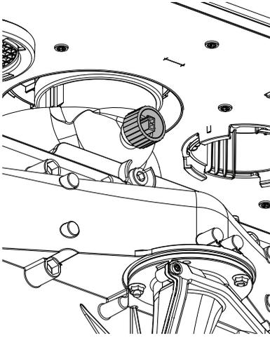
Figure 40: Flue gas Temperature Sensor S5
