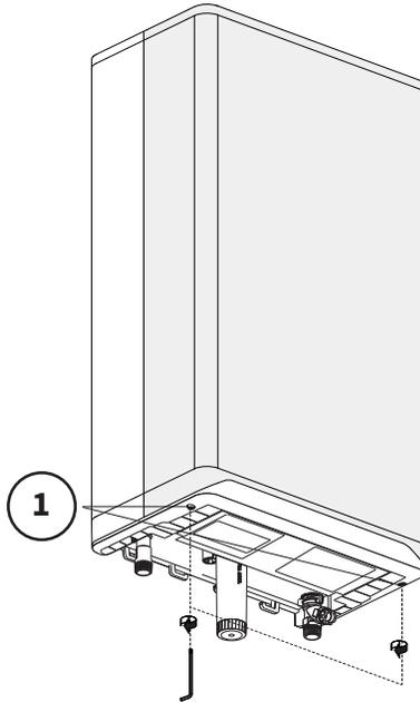
Figure 3: Loosen screws
