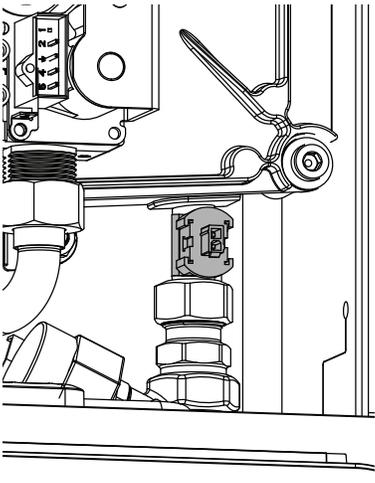
Figure 44: Domestic Cold Water Temperature Sensor S4
