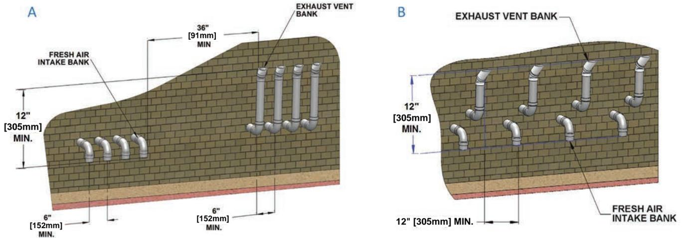
Figure 15: Sidewall vent termination - multiple vent piping configuration
