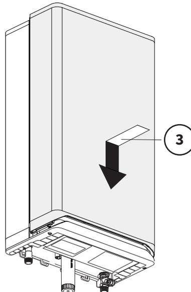
Figure 5: Positioning the frontpanel
