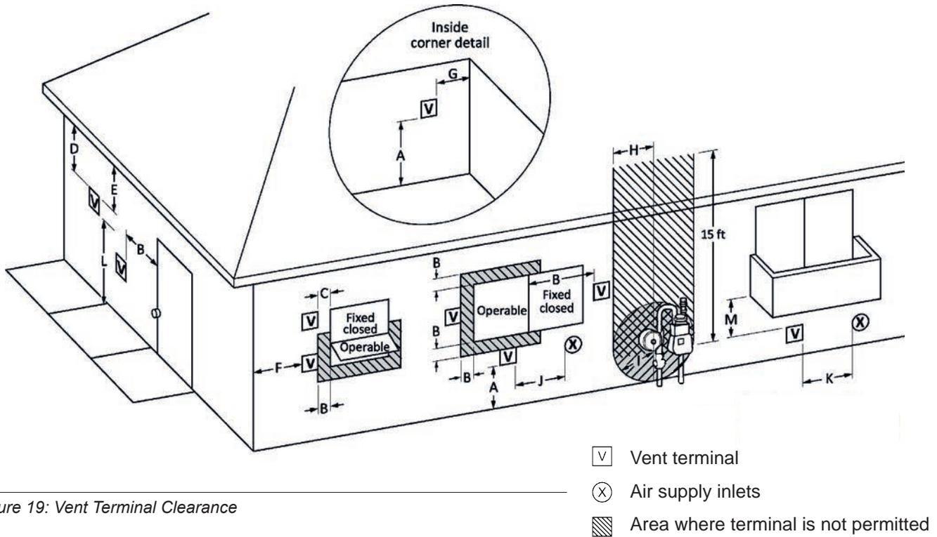
Figure 19: Vent Terminal Clearance
