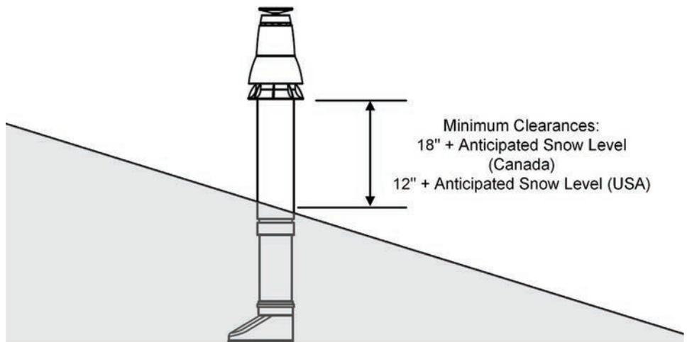
Figure 12: Vertical Concentric Termination - Single Kit
