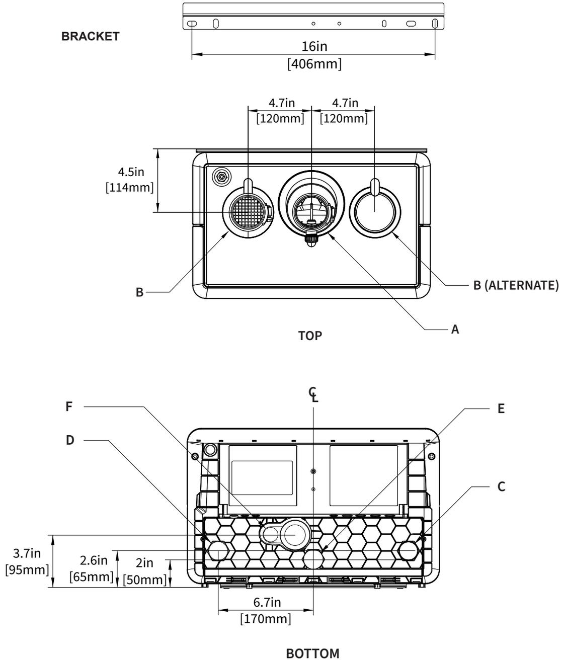
Figure 1b: Dimensions / Connections for Tankless Water Heater
