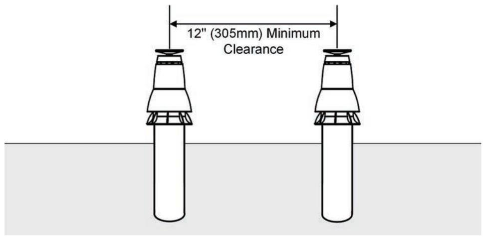
Figure 11: Vertical Concentric Termination - Two Kits
