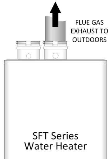
Figure 3: Basic exhaust vent assembly
