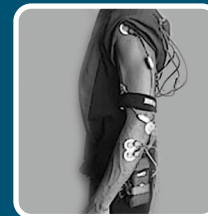
Illustration of test participant wired for electromyography
