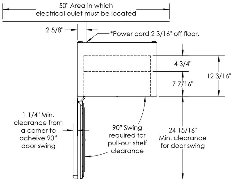
\* - Leg levelers can add 3/4" to these dimensions when fully extended.
