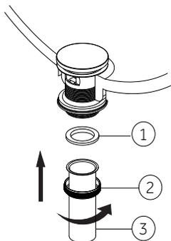
9. IMPORTANT: After installation is complete, remove the aerator from the faucet (2) to flush the water lines. Do not lose the gasket (1) in the aerator.
