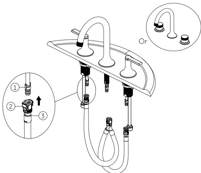
5. Make connections to water lines. Use 1/2" I. P. S. faucet connections (2) or use supply line coupling nuts (3) with 3/8" O. D. ball-nose riser (1). Use wrenches to tighten connections. Do not overtighten.
