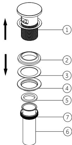
7. Place the washer (2) underneath the flange of the pop-up body (1). Slide the pop-up body (1) down through the drain hole on the vessel or basin. From underside, slide the washer (3 & 4) against the bottom of the vessel or basin, thread on the coupling nut (5) and tighten. Do not over tighten.
