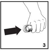
3. Visually inspect the fitting to ensure the grip ring, separator ring, and seal are in place, clean and, free of contaminants. Only original NIBCO yellow HNBR Bench PressG<sup>™</sup> seals are to be used.
