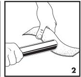
2. Prep pipe to a smooth and even surface with a fine grit sandpaper. The surface should be free of indentations, oil, and debris. Do not use engraved or stamped pipe. Indentations in the pipe may result in an improper seal. To avoid damage to the O-ring, the pipe must be free of burrs and sharp edges.
