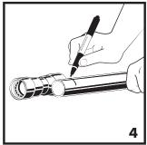
**4.** Mark the pipe to the proper insertion depth as indicated by the Insertion Depth Chart. Improper insertion depth may result in an improper seal.
