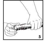
**5.** Fully insert the pipe into the fitting. For fittings with stops, insert the pipe to make contact with the fitting stop. For fittings without a stop, insert the pipe to a depth no less than the specified insertion depth. Improper insertion depth may result in an improper seal. If necessary, the O-ring may be lubricated with water. Never use oils or lubricants as these can degrade or damage the sealing element.
