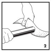
2. Prep pipe to a smooth and even surface with a fine grit sandpaper. The surface should be free of indentations, oil, and debris. Do not use engraved or stamped pipe. Indentations in the pipe may result in an improper seal. To avoid damage to the O-ring, the pipe must be free of burrs and sharp edges.
