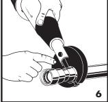
6. Ensure the proper press jaw is installed in the pressing tool. Squeeze the jaw arms to open the jaw set. Place open jaws around the fitting end and ensure the jaw is properly aligned with the contour of the fitting. When using the ring and actuator instead of jaws, use the correct size ring an appropriate actuator. See NIBCO Tool and Jaw Compatibility Matrix for approved tools and jaws.
