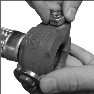
1. Loosen the nut of the Style 108 Coupling. Remove the Style 108 Coupling from the end of the Series AH1-CC, AH2-CC, or AH2-CC-300 Flexible Hose.
