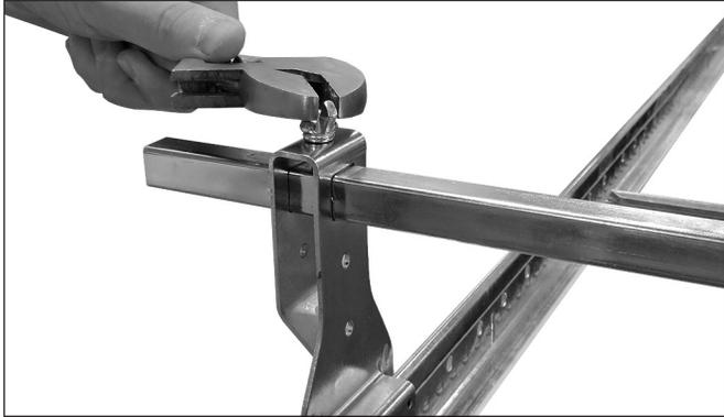
**FOR STYLES AB1 AND AB2 BRACKETS ONLY:** For adjustment purposes, the wing screw on top of the end bracket assembly can be loosened to allow the end bracket to slide on the square bar. Tighten the wing screw on top of the end bracket assembly to a torque of 36 inch-lbs/4 N•m (approximately ½ to ¾ of a turn past hand-tight) to secure the end bracket to the square bar.
