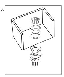
4. Screw in the 3 screws into the Mounting Ring. Fully tighten all 3 screws. The flange is now secured to the sink.
