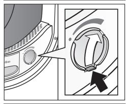
If you are not using a fragrance flacon: Push the tab down completely (see arrow) so that the socket is closed. Otherwise, lint will accumulate here.
