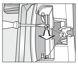
Use the screwdriver or pointed pliers to guide first one then the other rod
