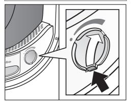
Open the cover using the tab until the tab is right at the top as shown.
