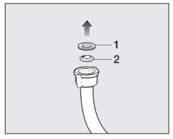
■ Remove the rubber seal **1** from the connector.
