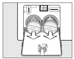
■ Remove the drain filters completely.
