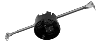
4" round new work non-metallic box with hanger bar assembly 4" diameter x 2-3/16" (102mm x 56mm)
