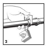
**2.** If you are unable to obtain complete contact with the copper fitting or see any kind of gap between the gauge and the fitting at the top of the gauge (arch), the crimp has not been successful.
