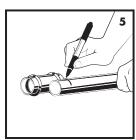
5. Mark the tube with the proper insertion depth using a NIBCO insertion depth tool and a permanent marker. Improper insertion depth may result in an improper seal.
