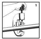
1. Select clean, undamaged copper tube and cut to desired length using a wheel type cutter. Do not use a hacksaw or reciprocating saw. Do not crimp over any etched print on the tube.
