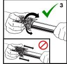
3. Polish the end of the tube with an abrasive pad (such as Scotch-Brite® 7447 Maroon by  $3M^{\scriptsize @}$  or equivalent) in a radial manner for 5-7 seconds. Do not polish axially. The tube end must be free from any oxidation, dirt, debris, and any imperfections. The surface of the tube should be shiny and bright. If sandpaper or emery cloth must be used, polish with 360-400 grit.
