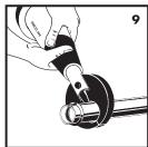
9. Before pressing, make sure that the tube is inserted to the proper depth in the fitting. Start the pressing process. Refer to the tool operating instructions for proper tool operation. Squeeze jaw arms to open jaw set and remove from the pressed tube fitting assembly.
