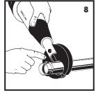
8. Ensure that the proper pressing jaws are installed in the pressing tool and squeeze jaw arms to open jaw set. Place open jaws around the fitting end and ensure the jaw is properly aligned with the contour of the fitting. For sizes 1-1/8" and above, the jaw has a pipe side and bead side orientation
