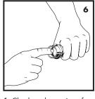
6. Check each opening of the fitting to make sure that the seal is in place. Only original NIBCO gray HNBR seals are to be used. Do not use a fitting that does not have a visible seal.
