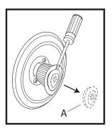
3. Remove handle (C) using screwdriver (B) as shown.
