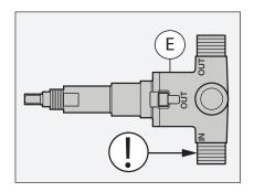
Secure stringer mounts on diverter valve (E) to wood blocking for support.
