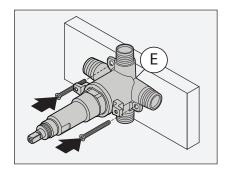
**Note:** Securing stringer mounts is necessary for applications where PEX, or other non rigid tubing, is used to install diverter valve.
