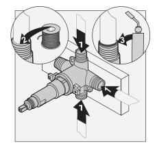
**Optional:** Apply plumber tape to male IPS threads on the inlet and outlet ports of diverter valve. Install 1/2"-14 NPT copper fittings to the inlet and outlet ports. Connect outlets to desired accessories.
