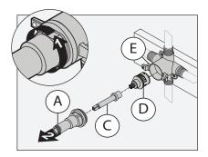
Note: Spacer (B) will be seated inside cap assembly (A).
