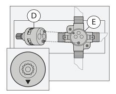
Align spindle extender (C) with broach on cartridge (D). Install spindle extender (C) and cap assembly (A) to cartridge (D). Secure cap assembly (A) by turning clockwise.
