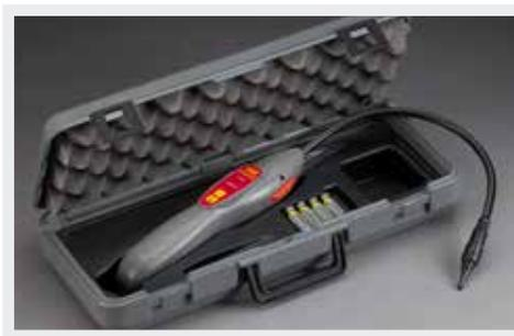
Many countries are now adopting laws that ban the use of refrigerants for system testing. The YELLOW JACKET H<sub>2</sub> was developed for the H<sub>2</sub> (95% nitrogen and 5% hydrogen) tracer gas mixture.
