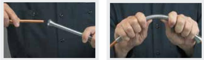
Spring benders slip over soft copper and aluminum tubing during bending to help prevent tube collapse.
