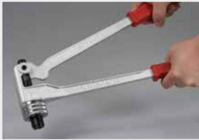
With long handles for comfortable leverage, easily expand 5/16" to 1-1/8" O.D. soft copper and aluminum tubing in seconds. Select from nine expander heads to attach to the front of the handles.
