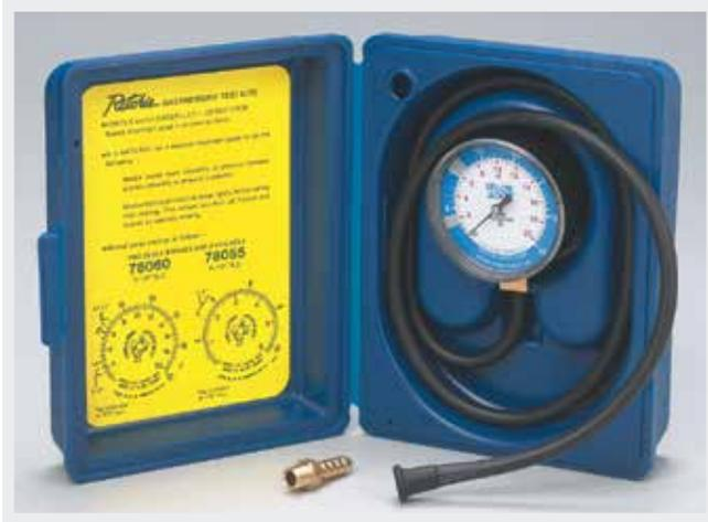
Easier to use than a manometer, this compact kit helps you accurately set manifold pressure for natural or L.P. gas.
