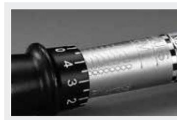
The N-M and foot-pound (FT-LB) scales are marked on the barrel of the wrench for easy and permanent reference.
