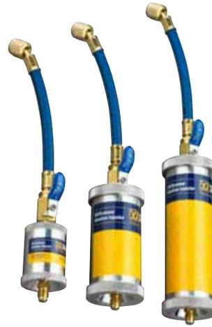
Body and cap are rugged aluminum with an "O" ring seal. 1/4" Male fitting at one end with Schrader. A ball valve for control on other end with a short length of hose. Valve depressor in 1/4" Female end. 600 psi working pressure.
