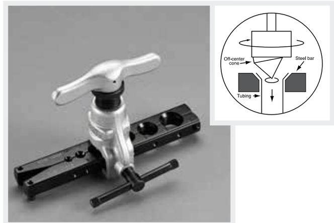
Off-center hardened steel cone with 45° flare produces a rolling action for uniform flare walls without galling in 3/16" to 3/4" O.D. tubing.
