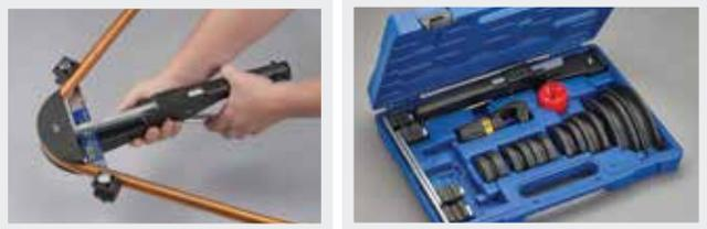
Easy one hand bending of 1/4" to 7/8" soft copper and soft aluminum. Hard copper must be annealed before bending.
