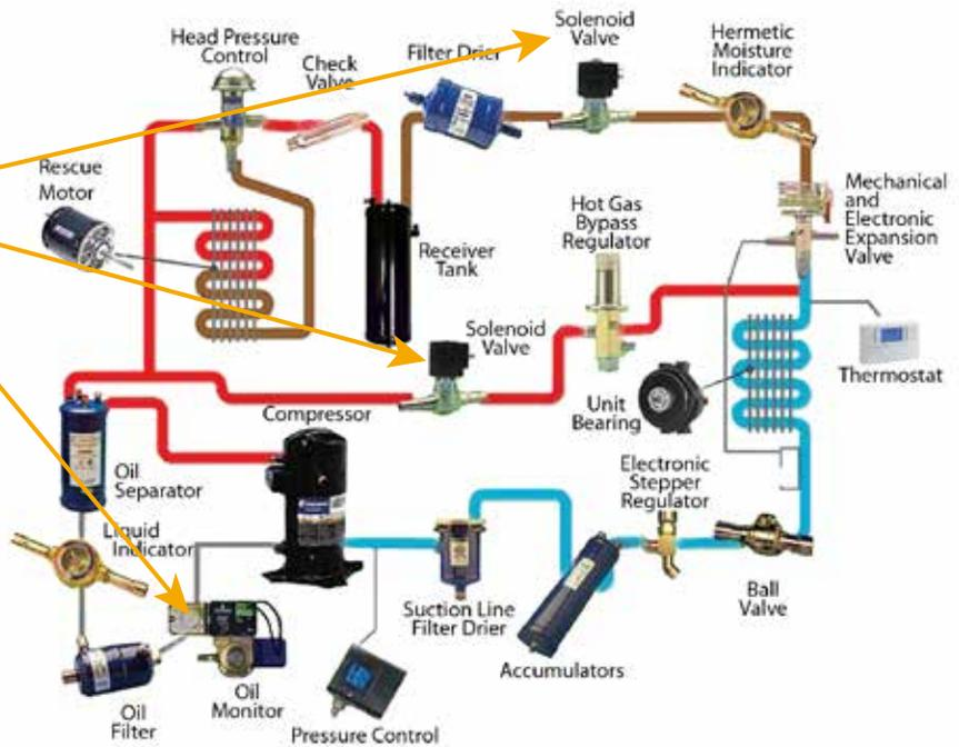
To optimize recovery, simply remove the solenoid coil from all normally closed valves – refrigerant control valves, hot gas defrost valves, reversing valves, etc. Then apply the **YELLOW JACKET®** solenoid magnet to each valve to speed up recovery and evacuation.
