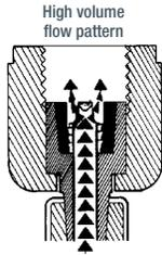
The "Adjust-a-Valve" valve core depressor easily opens out-of-tolerance Schrader valves. Simply adjust height with needle nose pliers. Designed for repeat usage; replacement is convenient.
