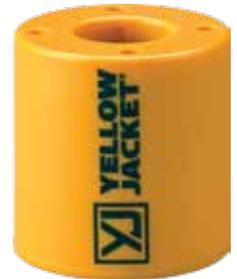
The **YELLOW JACKET®** Solenoid Valve Service Magnet is the quickest and easiest way to manually operate solenoid valves. It works by magnetically lifting the stem assembly and plunger to actuate the valve during service.
