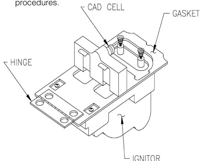
**Figure 8-8: Cad Cell Location**
