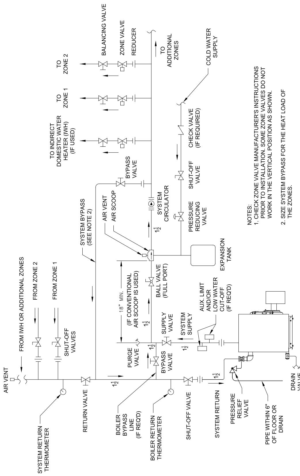
**Figure 3-3: Recommended Water Piping for Zone Valve Zoned Heating Systems**
