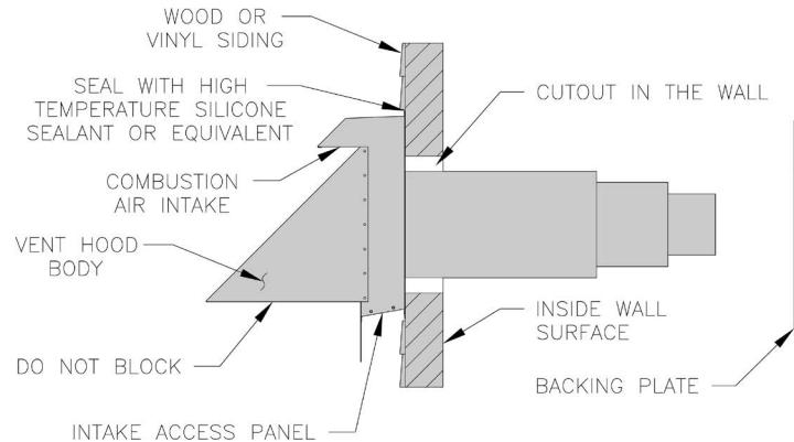
**Figure 5-4: Vent Hood Body Installation**
