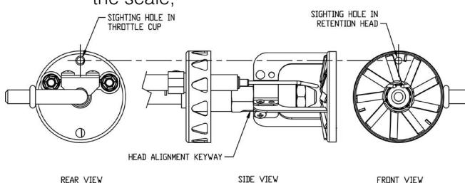
**Figure 8-4: Retention Head/Throttle Cup Alignment**
