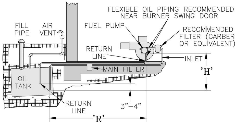
**Figure 7-4: Two Pipe Oil Lines**
