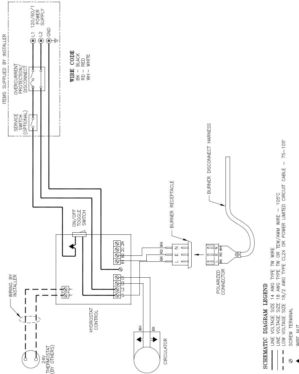
**Figure 6-1: Schematic Wiring Diagram**
