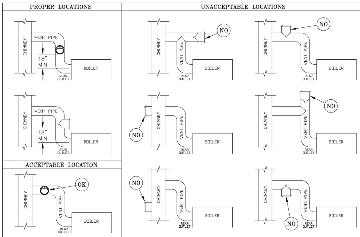
Figure 4-2: Proper and Improper Locations of Draft Regulator
