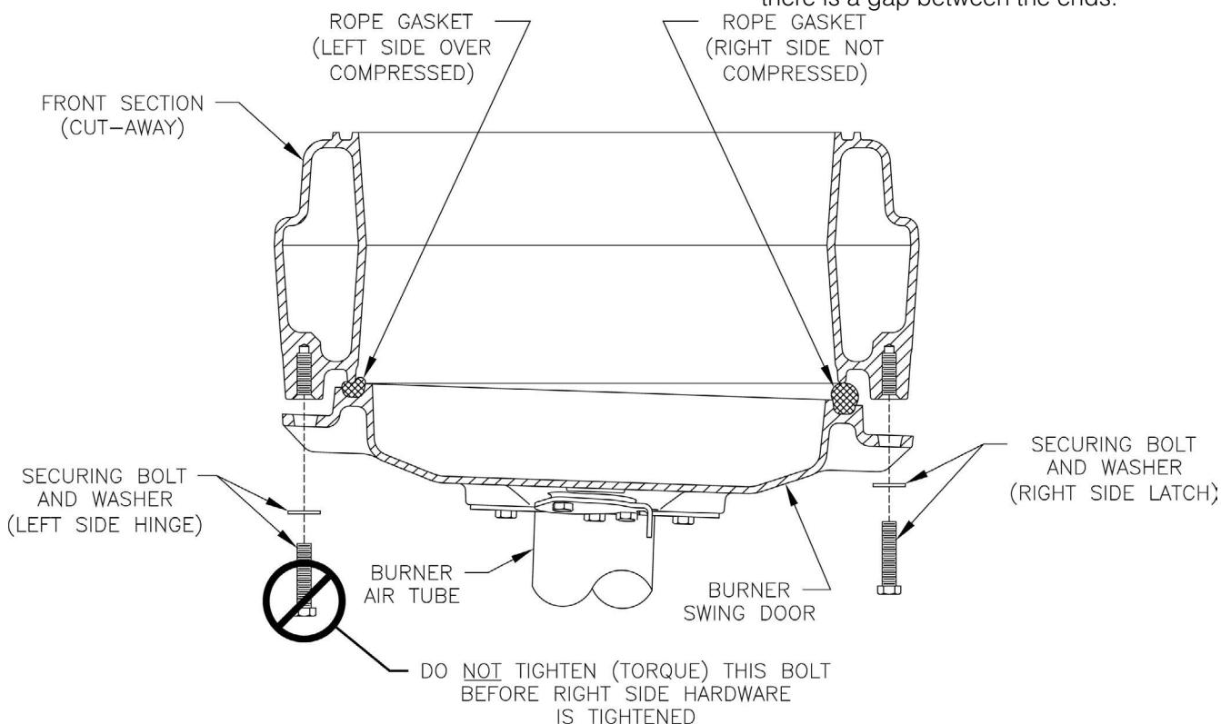
Figure 2-4: Top View - Burner Swing Door Fully Closed but Not Properly Secured or Sealed
