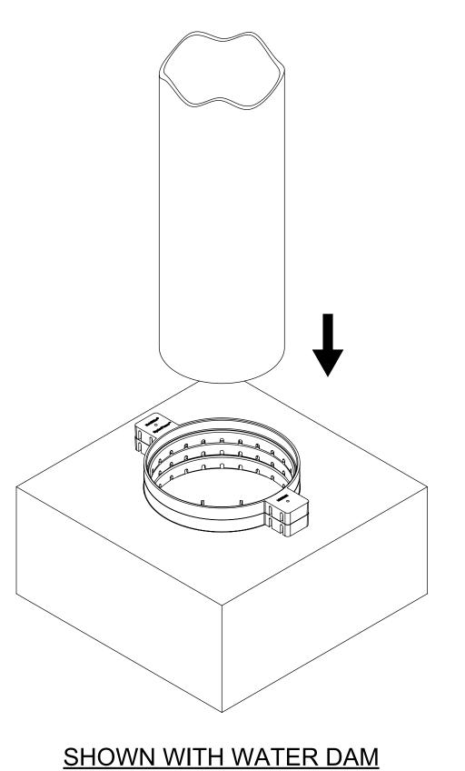
STEP #6 (INSTALL PENETRANT FROM THE TOP)
