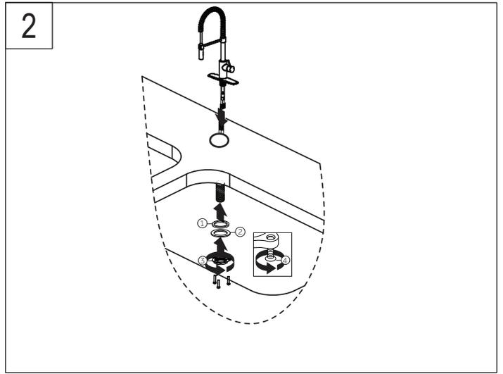
2. Thread the faucet through the mounting hole. Secure to sink by rubber washer (1), steel washer (2), tighten the lock nut (3), and mounting screws (4). Do not over tighten.
