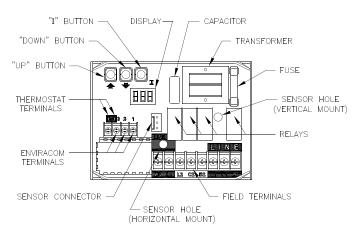
Figure 11-2: Intelligent Oil Boiler Control
