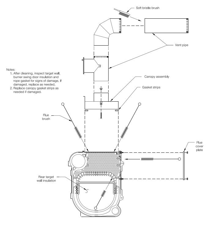
Figure 13-1: Cleaning of Boiler Flueways
