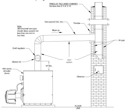
Figure 7-1: Recommended Vent Pipe Arrangement and Chimney Requirements
