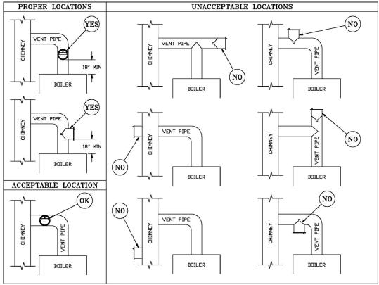
Figure 7-2: Proper and Improper Locations of Draft Regulator
