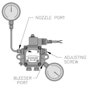
Figure 11-1: Adjusting Fuel Pump Pressure
