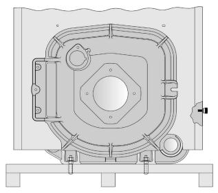
Figure 4-1: Packaged Boiler Removal from Skid
