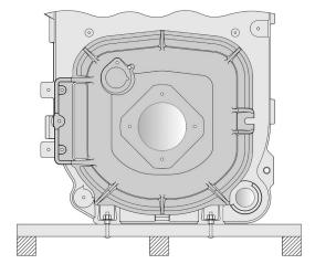
Figure 3-1: Knockdown Boiler Removal from Skid
