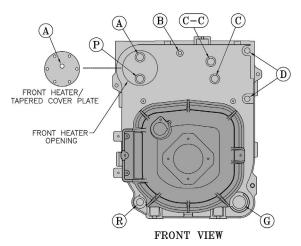
Figure 3-3: Boiler Tapping Locations and Usage (Knockdown Boilers Only)
