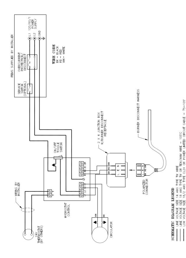
Figure 8-3: Schematic Wiring Diagram, Water Boiler, Hydrolevel Hydrostat (All Burners)
