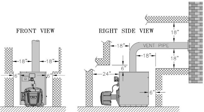
Figure 2-1: Minimum Installation Clearances To Combustible Materials (Inches)
