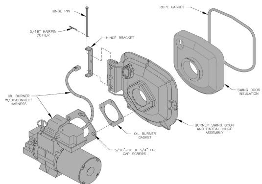
Figure 3-5: Oil Burner Installation (Beckett Burner Shown)
