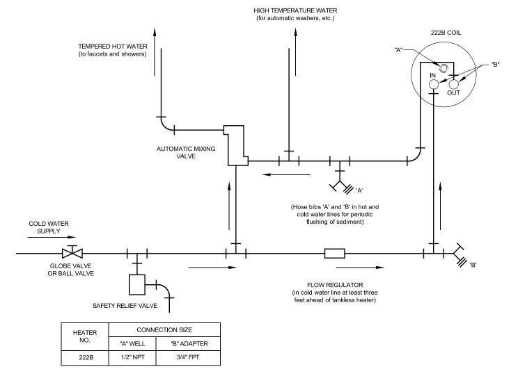
Figure 6-1: Schematic Tankless Heater Piping
