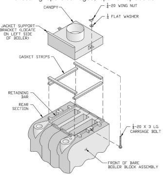
Figure 3-2: Boiler Canopy Installation
