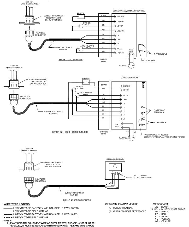
Figure 8-4: Schematic Wiring Diagrams For All Burner Options w/Various Oil Primary Controls
