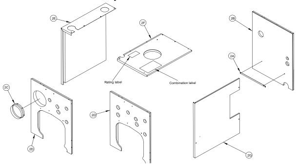
Figure 3-4: Knockdown Boiler Jacket Assembly
