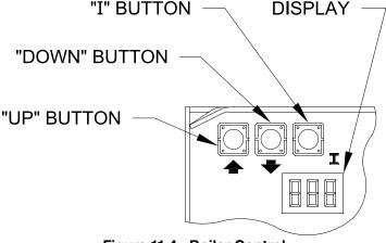
Figure 11-4: Boiler Control Key Function & Orientation
