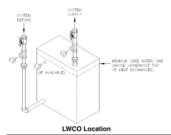
Select the appropriate size tee using the LWCO manufacturer's instructions. Often, the branch connection must have a **minimum** diameter to prevent bridging between the probe and the tee. Also, the run of the tee must have a minimum diameter to prevent the end of the probe from touching or being located too close to the inside wall of the run of the tee.
